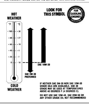
As shown in the chart, SAE 5W-30 is best for your vehicle. However, you can use SAE 10W-30 if it's going to be 0°F (-18°C) or above. These numbers on an oil container show its viscosity, or thickness. Do not use other viscosity oils, such as SAE 20W-50.
